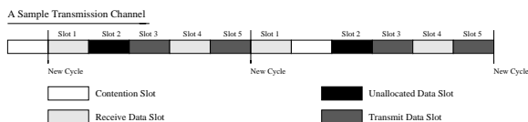
Figure 1: GAMMA: In this example there are five data slots in a cycle; however, the interval between consecutive contention slots is six. Because of this difference, the number of contention slots per cycle varies; the first cycle does not have a contention slot while the second cycle has one. A data slot may be used to transmit or receive data or it may be unallocated.
