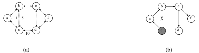
Figure 5. The third part of LORA-3 not always triggers the generation of an update message: (a) network topology, and (b) the new source tree of node c after processing the failure of link (c, b) .
